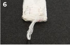
Repeat on the other site. Fold so that the width of the canopy is the same from the top to the bottom. Fold lines in double Z configuration as shows **figure 5**. Secure each with elastic band.
