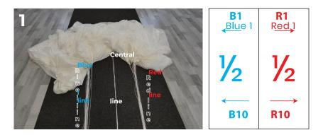
Divide canopy in to two parts, each should start with number 1 and end with number 10. Lines must be separated in to left main (blue) lines, central line and right main (red) lines.
