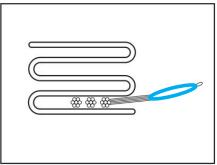
Stew the canopy in a Z configuration (**figure 7**) so that the skirt is atop the folds in the inner container. Close inner containers flaps with rubber closing loop attached to the one of the flaps. Make a final loop with left lines and secure it with closing loop. Make sure that the whole line jacket is out of the inner container as shows **figure 8**.
