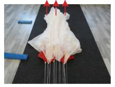
Make sure that the lines are not entangled by grabbing first two main lines next to the central line (first to the left and firs to the right) on the risers, and slowly guide them to the canopy. The should go separately all the way from the riser to the canopy. Check the numbers on the canopy. Number 1 should be facing up on the left and right.
